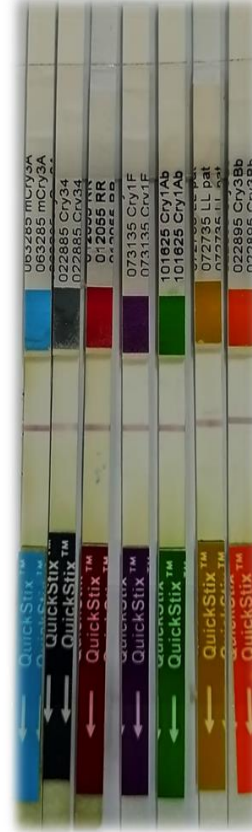
Fig.5 Detection of maize samples by LFST
